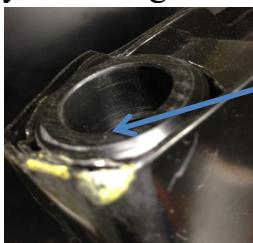
Depending on your tailgate the delrin (black piece) with Beveled edge could be installed inside the cup pocket or like it is shown – Ensure it's installed flush or just below flush of the tailgate
