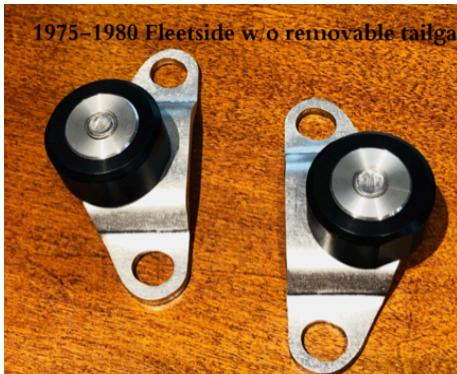
Pre-check to ensure proper installation. Test fit the female delrin bearing on both sides. If it goes in tight it will be very difficult to install the trunnion bracket (stainless) ball and will be tight while opening and closing the tailgate. You could sand the edges of the Delrin bearing (black parts) to make it fit better, tight but not to tight. Go slow and it just might need to be sanded a little more, the key is that you don't want the delrin (black part) to spin at all. Continue to check
