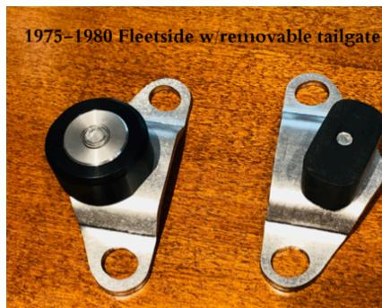
Pre-check to ensure proper installation. Test fit the female delrin bearing on both sides. If it goes in tight it will be very difficult to install the trunnion bracket (stainless) ball and will be tight while opening and closing the tailgate. You could sand the edges of the Delrin bearing (black parts) to make it fit better, tight but not to tight. Go slow and it just might need to be sanded a little more, the key it that you don't want the delrin (black part) to spin at all. Continue to check
